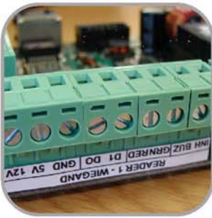
Full Wiegand support includes Red LED, Inhibit buzzer and anti-tamper switch
